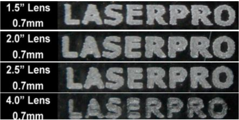
Engraving effects achieved with the different lenses
